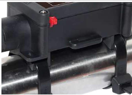
2: Two removable legs for fitting on pipes, providing a 10 mm offset from the tube. Ideal and economical for applications with low insulation thickness and pipe temperature below 100°C. Clamping on metal or PVC piping can be made by nylon tie or metal clamp (These tabs are included as standard).
