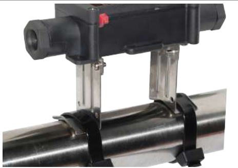
3: One stainless steel bracket, for offset mounting on piping, allowing the enclosure to be locked in after the insulation and its protection have been installed. Allow an insulation thickness of 50 mm, and can be used on hot pipes. Clamping on metal or PVC piping by nylon tie or metal clamp. (Legs available as an accessory.)
